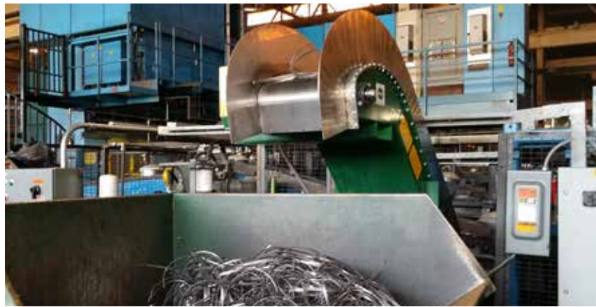
MPI built the "SCRAPINATOR" 1200 series Beltless Magnetic Conveyor (BLM) for a large stamping customer.
